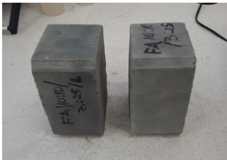
Fig. 5 - Shelled compressed earth block of High carbon fly ash, soil and cement
